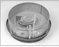
If flammable vapors accidentally enter the combustion chamber, the arrestor is designed so flames burn off the top surface and can not escape down through the arrestor.
