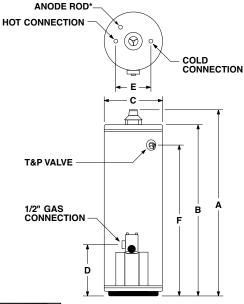
\*Location for optional top-mounted T&P Valve if ordered from factory.
