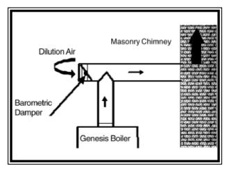
Figure 5-3 - Masonry Chimney
