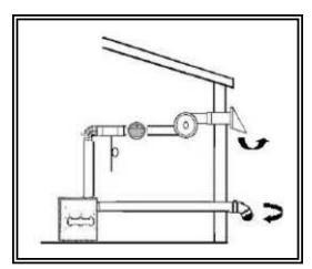
Figure 5-16 Extended Horizontal Direct Venting See Table M for Extended Horizontal Direct Venting
