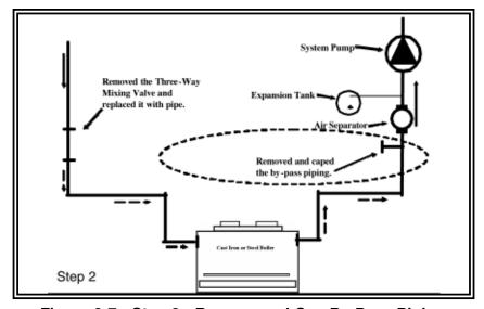
Figure 9-7 - Step 2 - Remove and Cap By-Pass Piping
