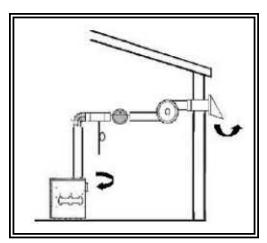
Figure 5-15 Extended Sidewall Venting See Table L for Extended Sidewall Venting
