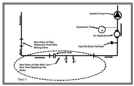
Figure 9-8 - Step 3 - Remove Old Cast Iron Boiler
