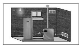
Figure 3-2 Air for Combustion (Through the Wall)
