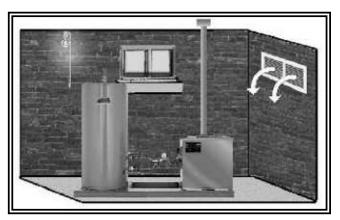
Figure 3-5 Alternate Air for Combustion (Through the Wall)
