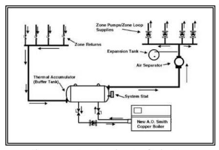
Figure 9-12 - Zone Pumping - Low/Varied Flow System With Horizontal Thermal Accumulator
