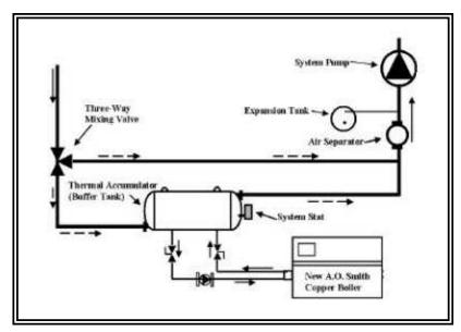
Figure 9-11 - Low/Varied Flow System With Horizontal Thermal Accumulator
