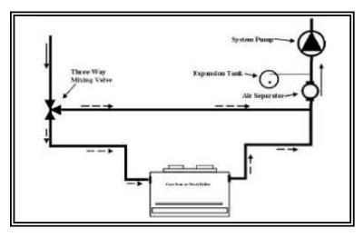
Figure 9-5 - System with Three-Way Mixing Valve
