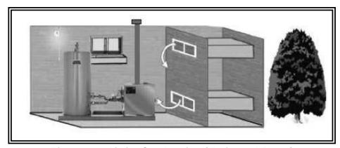
Figure 3-4 Air for Combustion (Horizontal Ducts)
