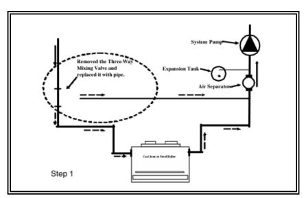
Figure 9-6 - Step 1 - Removing Mixing Valve
