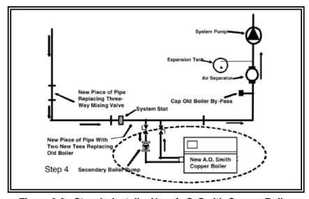
Figure 9-9 - Step 4 - Install a New A. O. Smith Copper Boiler
