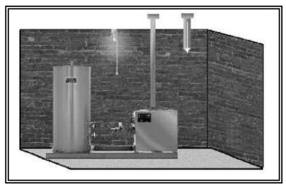
Figure 3-6 Alternate Air for Combustion (Vertical Duct)
