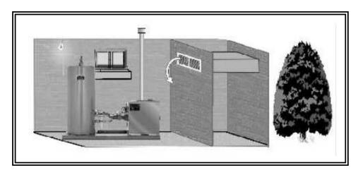
Figure 3-7 Alternate Air for Combustion (Horizontal Duct)
