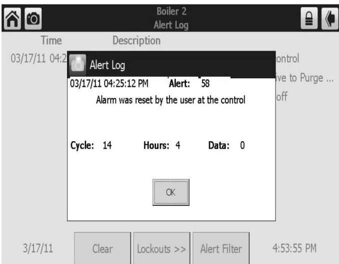
FIGURE 65. CONTROL EXPANDED ALERT DETAIL
