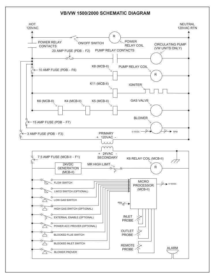
FIGURE 1 - SCHEMATIC DIAGRAM
