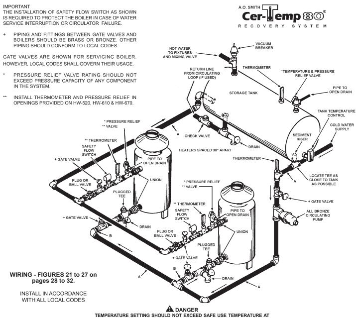
TEMPERATURE SETTING SHOULD NOT EXCEED SAFE USE TEMPERATURE AT FIXTURES. SEE TANK TEMPERATURE CONTROL WARNING ON PAGE 11. IF HIGHER PREHEAT TEMPERATURES ARE NECESSARY TO OBTAIN ADEQUATE BOOSTER OUTPUT, ADD AN ANTI-SCALD VALVE FOR HOT WATER SUPPLIED TO FIXTURES.
