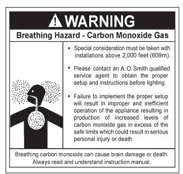
Rated inputs are suitable up to 2000 feet (610 m) elevation. Consult the factory for installation at altitudes over 2000 feet (610 m).
