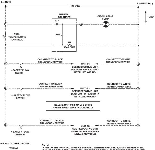
WIRING ——— BY FACTORY ----- BY INSTALLER IF ANY OF THE ORIGINAL WIRE, AS SUPPLIED WITHTHE APPLIANCE, MUST BE REPLACED, IT MUST BE REPLACED WITH TYPE 105°C WIRE OR EQUIVALENT, EXCEPT FOR THE FLAME SENSOR AND IGNITION CABLE (I.I.D. UNITS ONLY) WHICH ARE 250°C AND WIRES CONNECTED TO THE COIL PROTECTOR WHICH ARE 200°C.
