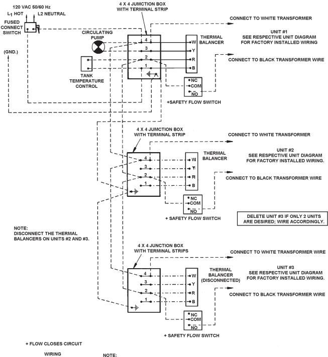
IF ANY OF THE ORIGINAL WIRE, AS SUPPLIED WITH THE APPLIANCE, MUST BE REPLACED, IT MUST BE REPLACED WITH TYPE 105°C WIRE OR ITS EQUIVALENT, EXCEPT FOR THE FLAME SENSOR AND IGNITION CABLE (I.I.D. UNITS ONLY) WHICH ARE 250°C AND WIRES CONNECTED TO THE COIL PROTECTOR WHICH ARE 200°C.
