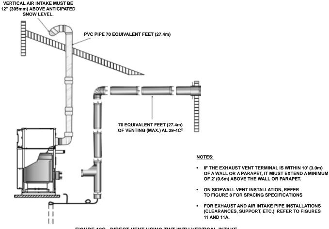
FIGURE 12C. DIRECT VENT USING TWT WITH VERTICAL INTAKE.
