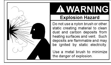
Qualified serviceman should follow this procedure when the boiler's intake and exhaust piping need cleaning:
