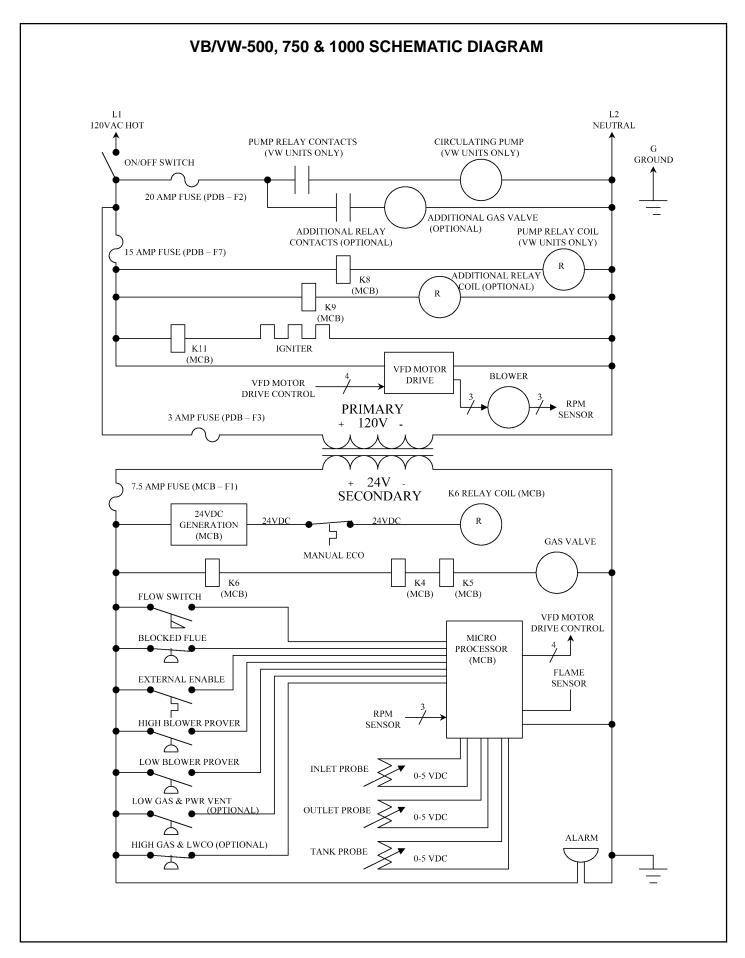
FIGURE 17 - SCHEMATIC DIAGRAM
