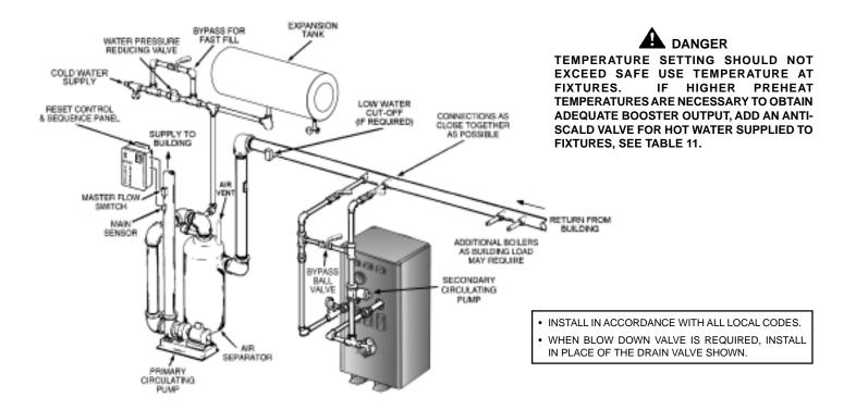
FIGURE 13. TYPICAL PRIMARY, SECONDARY PIPING.
