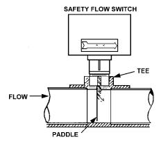
FIGURE 6. WATER FLOW SWITCH.
