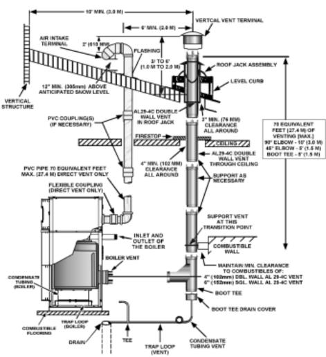
FIGURE 12A. DIRECT VENT VERTICAL.
