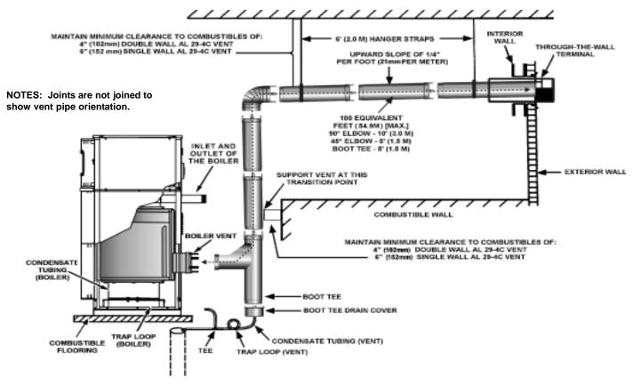
FIGURE 11A. HORIZONTAL THROUGH THE WALL TERMINATION (TWT).
