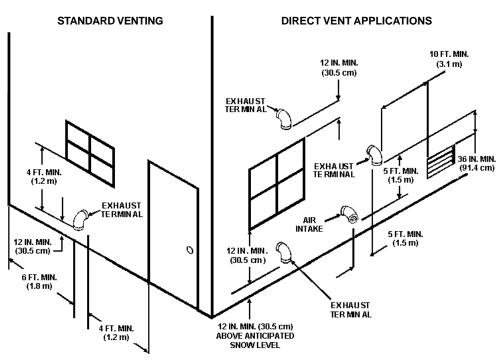
Figure 5. Vent Termination Installation Clearances
