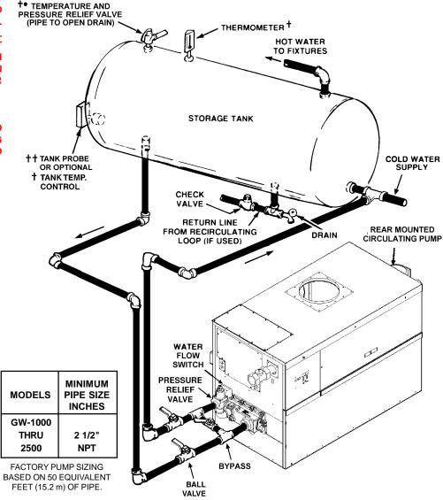
Figure 11. Single boiler with horizontal tank.
