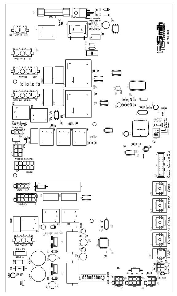
Figure 17. CCB CENTRAL CONTROL BOARD
