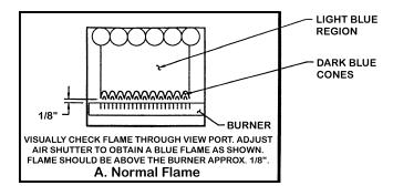
Figure 22. Normal Flame Characteristics
