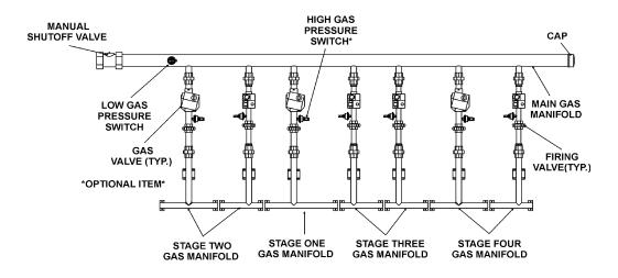
Figure 14. GB/GW 1000 - 2500 Gas Manifold Assembly Diagrams.
