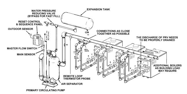
Figure 10. Single or Multiple Boiler Installation Diagram
