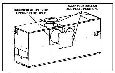
Figure 4. Switching from Vertical to Horizontal Venting.
