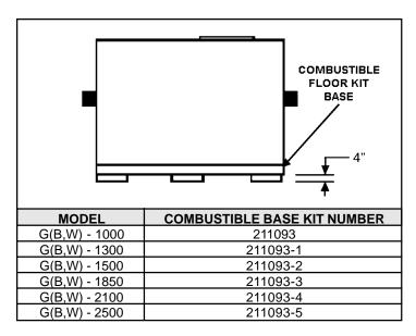
Figure 3. Boiler on Combustible Floor Base and Kit Numbers.
