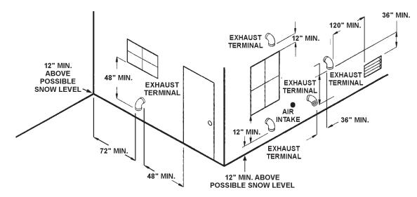
FIGURE 18. VENT TERMINATIONS AND INSTALLATION CLEARANCES
