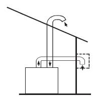
FIGURE 13. DIRECT VENT HORIZONTAL/VERTICAL TERMINATION
