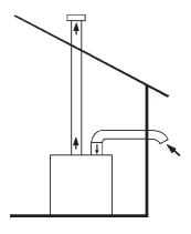
FIGURE 14. DIRECT VENT VERTICAL/HORIZONTAL TERMINATION
