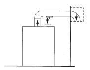
FIGURE 11. SINGLE PIPE HORIZONTAL TERMINATION
