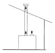
FIGURE 10. SINGLE PIPE VERTICAL TERMINATION
