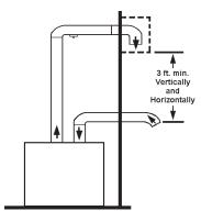
CAUTION Direct venting into dead air spaces such as alleys, atriums and inside corners can cause recirculation of flue gases. Recirculation of flue gases will cause sooting, premature failure of the heat exchanger and icing of the combustion air intake during severe cold weather. prevent the recirculation of flue gases, maintain as much distance as possible between the combustion air intake and the exhaust vent terminal.
