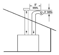
FIGURE 15. DIRECT VENT VERTICAL TERMINATION AND MINIMUM CLEARANCES
