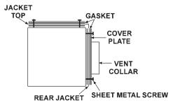
FIGURE 17. REAR VENT INSTALLATION
