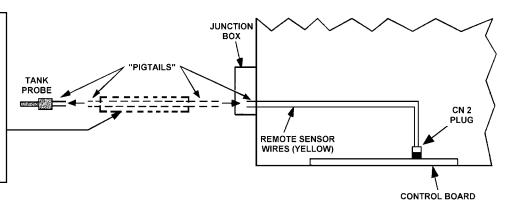
Figure 5. Tank Probe Installation
