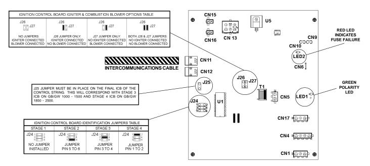
Figure 2. Jumper Configurations for Ignition Control Board.
