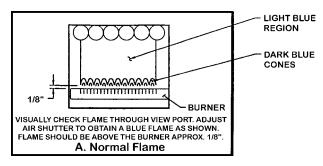
Figure 6. Burner Flame Characteristics
