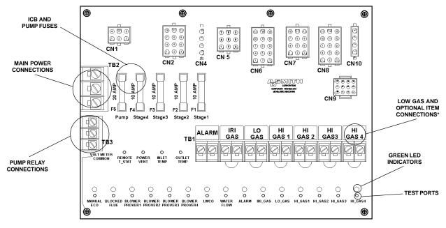
Figure 3. Interface Board Components.
