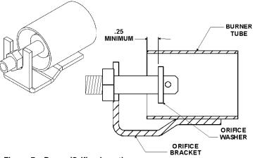
Figure 7. Burner/Orifice Insertion
