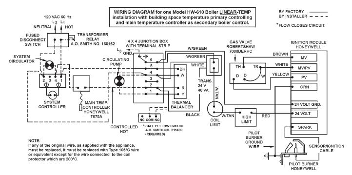
TYPICAL WIRING DIAGRAM (IID NATURAL GAS) FOR SINGLE BOILER <u>LINEAR</u>-TEMP® INSTALLATION FOR CANADIAN MODELS FIGURE 12
