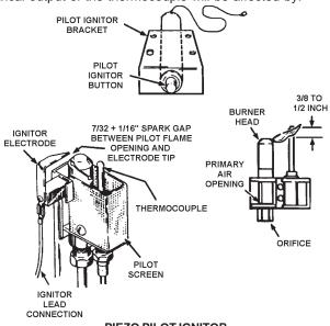
PIEZO PILOT IGNITOR FIGURE 43A
