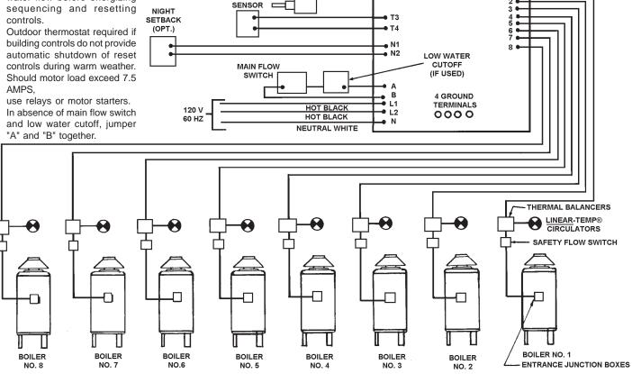
Boilers and Secondary Circulator areControlled by <u>Dual Bulb, Dual Switch Controller</u> Staging and Outdoor Reset of Main Water Temperature
