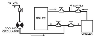
SCHEMATIC SHOWING PROPER PIPING ISOLATION
