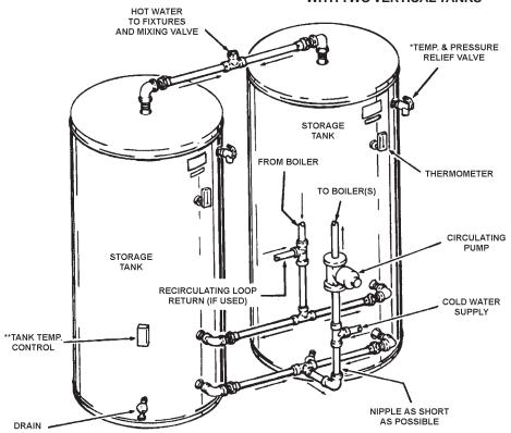
NOTE: CIRCULATOR AND PIPE SIZE TO BE SELECTED FROM THE CER-TEMP 80 DIAGRAM FROM THE BOILER MODEL TO BE INSTALLED.
