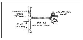
FIGURE 13. GAS PIPING WITH FLEXIBLE CONNECTOR.
