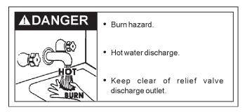
The temperature-pressure relief valve must be manually operated at least once a year.
