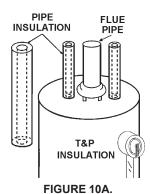
Fit pipe insulation over the incoming cold water line and the hot water line. Make sure that the insulation is against the top cover of the heater. Fit T & P valve insulation over valve. Make sure that the insulation does not interfere with the lever of the T & P valve.
