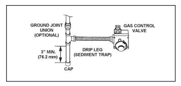
FIGURE 13. GAS PIPING WITH FLEXIBLE CONNECTOR.
