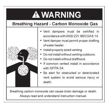
VENT DAMPERS - Any vent damper, whether it is operated thermally or otherwise must be removed if its use inhibits proper drafting of the water heater.
