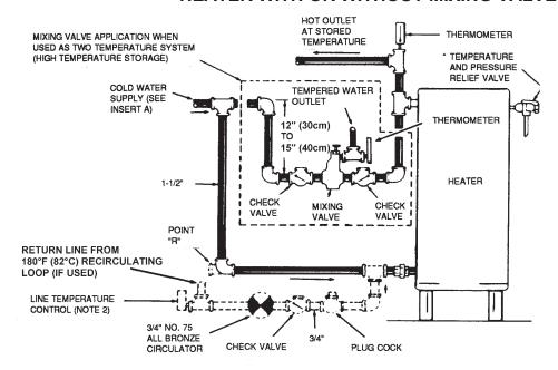
TEMPERATURE SETTING SHOULD NOT EXCEED SAFE USE TEMPERATURE AT FIXTURES. SEE WATER TEMPERATURE CONTROL WARNING ON PAGE 25. IF HIGHER PREHEAT TEMPERATURES ARE NECESSARY TO OBTAIN ADEQUATE BOOSTER OUTPUT, ADD AN ANTI-SCALD VALVE FOR HOT WATER SUPPLIED TO FIXTURES.
