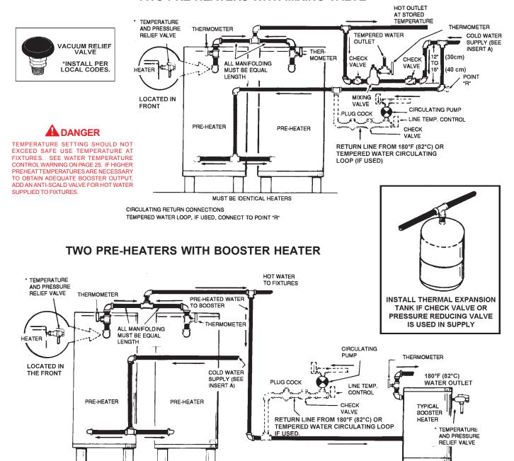
CAUTION: IF BUILDING COLD WATER SUPPLY HAS A BACKFLOW PREVENTER, CHECK VALVE OR WATER METER WITH CHECK VALVE, PROVISIONS FOR THERMAL EXPANSION OF WATER IN THE HOT WATER SYSTEM MUST BE PROVIDED.
