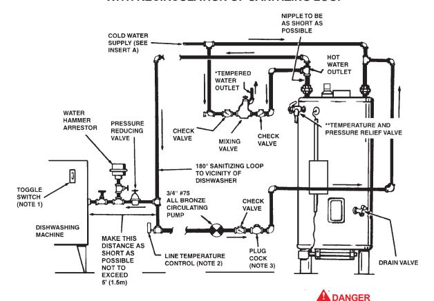
NOTE 1: TOGGLE SWITCH CONTROLS 180°F (82°C) WATER CIRCULATION. INSTALL ON OR CLOSE TO DISHWASHING MACHINE. TOGGLE SWITCH MUST BE CLOSED (ON) DURING THE RINSE OPERATION AND OPEN (OFF) WHEN DISHWASHER IS NOT OPERATING OR WHEN ON LONG STANDBY.
