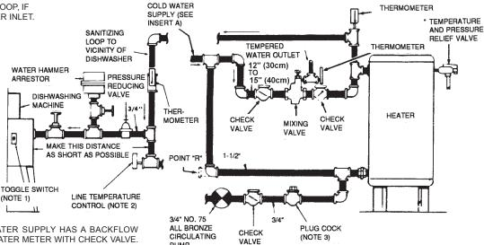
CAUTION: IF BUILDING COLD WATER SUPPLY HAS A BACKFLOW PREVENTER, CHECK VALVE OR WATER METER WITH CHECK VALVE. PROVISIONS FOR THERMAL EXPANSION OF WATER IN THE HOT WATER SYSTEM MUST BE PROVIDED.
