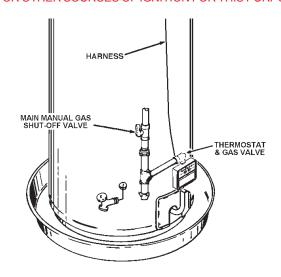
FIGURE 5 - GAS PIPING AND DIRT LEG INSTALLATION
