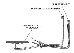
FIGURE 7-MAIN BURNER AND IGNITER ASSEMBLY - NATURAL GAS
