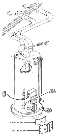
CONTROL SEQUENCE - HOT SURFACE DIRECT IGNITION Pre-purge seconds HSI Warm-up 20 seconds Ignition Activation Period 4 seconds Flame Recognition Period 1 second. Ignition Trial 4 seconds Interpurge 5 seconds Post-purge 5 seconds Retries 2 Reset from Lockout 1 hr. Flame Sensing (Nominal) HSI Off/Run Mode 4.0µ DC
