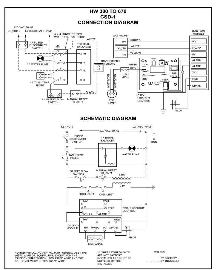
FIGURE 3. WIRING DIAGRAM
