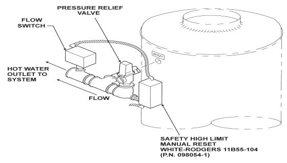
FIGURE 2. CSD-1 OUTLET MANIFOLD
