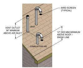
Figure 4-2 Vertical Termination of Air and Vent w/Rain Cap
