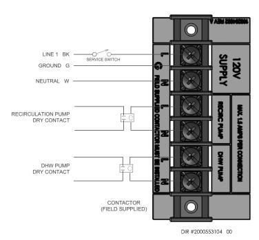
Figure 8-1B Line Voltage Field Wiring Connections - 208V
