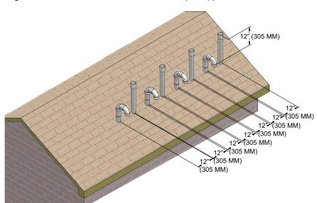
**Figure 4-4** Alternate Vertical Terminations with Multiple Appliances
