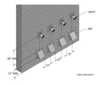
Figure 5-6 Direct Vent Terminations
