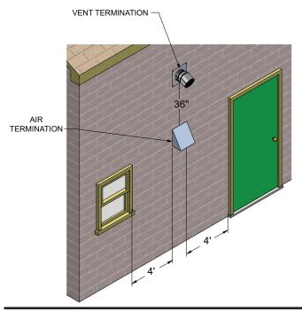
Figure 5-4 Clearance to Forced Air Inlets
