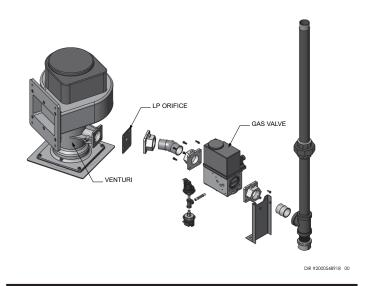
Figure 2-4 Installing Air Orifice Plate - Models 3000 & 4000
