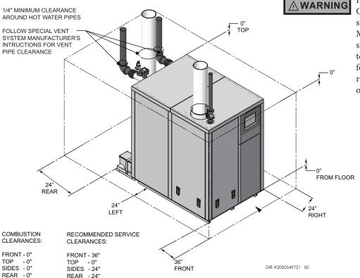
For alcove installations, CPVC, polypropylene, or stainless steel vent material MUST BE used in an alcove structure due to elevated temperatures. Failure to follow this warning could result in fire, personal injury, or death.
